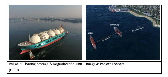
A LNG carrier shall supply LNG to the FSRU and will only stay 1-2 days to offload the LNG cargo. The LNG remains on the FSRU and is regasified to natural gas which is then pumped from the FSRU to the Powership via gas pipeline.
